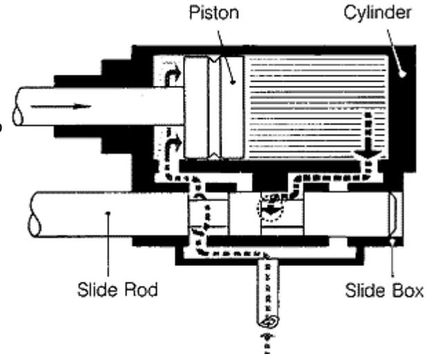
Just before the piston reaches the end of its travel, on the extreme right, the slide valve cuts off the steam from the boiler. This is the point, where the crank is at the limit of its movement and is known as Top-dead-centre or Bottom-dead-centre? Referring to the two possible geometric positions. The flywheel carries the crank over this critical position by the energy it has stored from previous power strokes.
