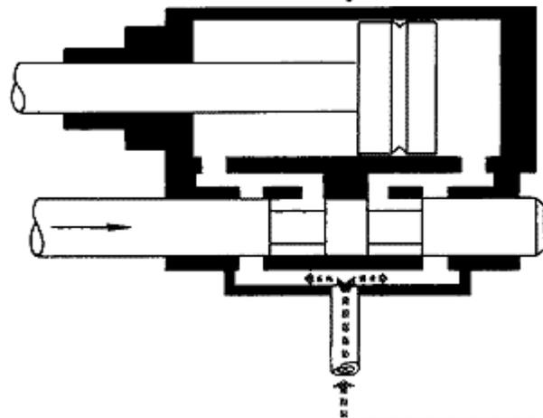
The slide valve continues to move in the same direction this time opening the inlet port to admit steam to the right hand side of the piston, again pushing the piston but now to the left, exhausting the steam through the left hand port. The whole cycle being repeated when the Dead centre is reached once more.
